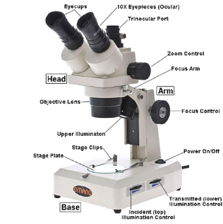
A typical stereomicroscope is as shown above. It has three key parts:
