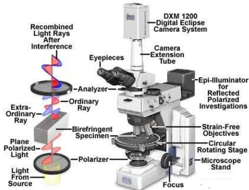
A typical polarizing microscope is as shown above.
